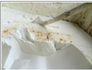
Lime Putty is the product that has historically been used as the binder in lime mortars. It has many names, and this sometimes causes issues, for example it can be known as Non Hydraulic Lime, Fat Lime or Air Dried Lime. It is made when quicklime is slaked with enough water to make a liquid and then left to mature for 3 months+ into a cottage cheese like consistency.
